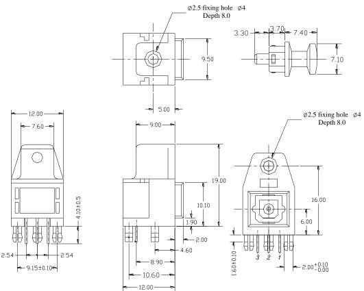
Note: 1.All dimensions are in millimeters. 2.General Tolerance :±0.3mm
