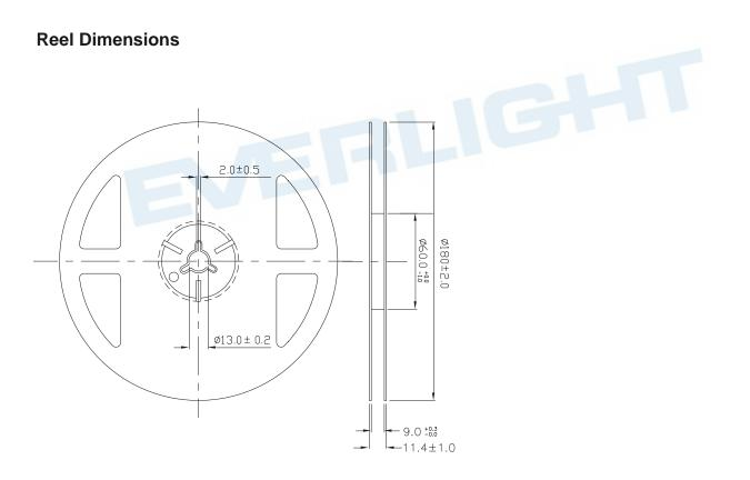
Note: The tolerances unless mentioned is  $\pm 0.1$ mm ,Unit = mm
