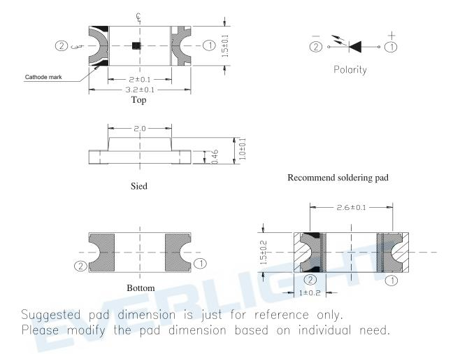
Note: Tolerances unless mentioned ±0.1mm. Unit = mm
