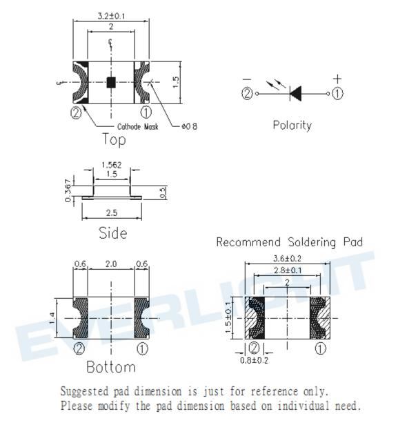
Note: Tolerances unless mentioned ±0.1mm. Unit = mm
