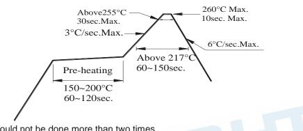
3.2 Reflow soldering should not be done more than two times.
