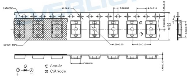
**Note:** The tolerances unless mentioned are ±0.1, unit=mm.
