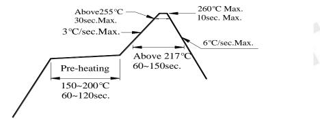
3.2 Reflow soldering should not be done more than two times.
