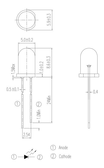
Note: Tolerances unless dimensions ±0.25mm
