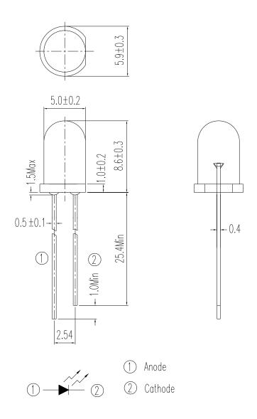
Note: Tolerances unless dimensions ±0.25mm
