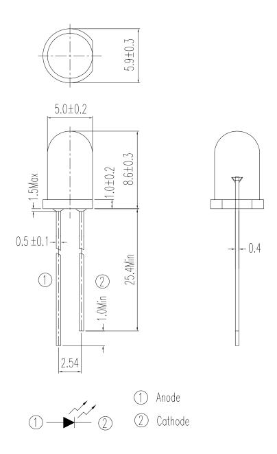
Note: Tolerances unless dimensions ±0.25mm
