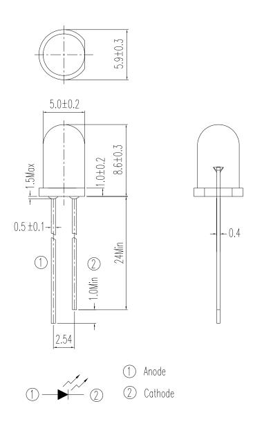
Note: Tolerances unless dimensions ±0.25mm
