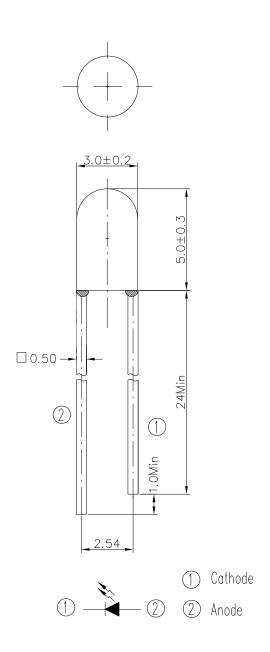
Note: Tolerances unless dimensions ±0.25mm
