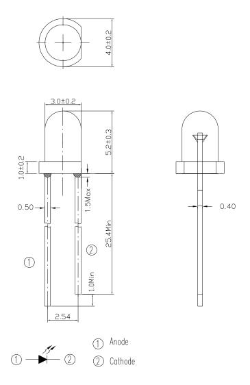
Note: Tolerances unless dimensions ±0.25mm
