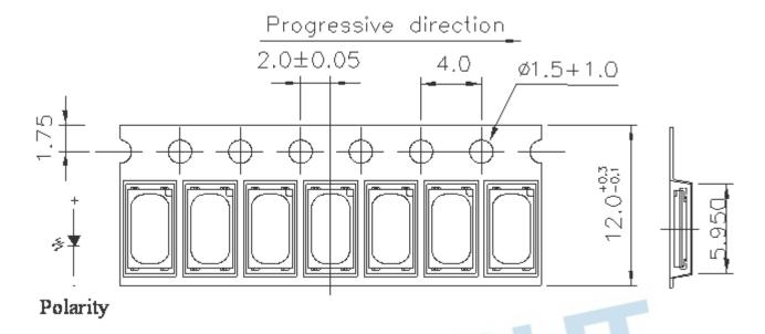
**Note:** 1.The tolerance unless mentioned is  $\pm 0.1$ , unit = mm.
