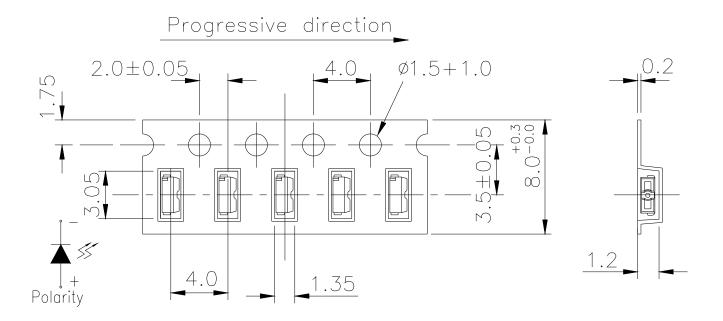
**Note:** 1. The tolerances unless mentioned is  $\pm 0.1$ mm; Unit = mm
