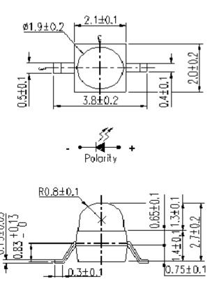
Note: The tolerances unless mentioned are ±0.1, unit=mm.
