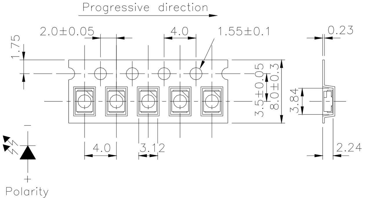
**Note:** Tolerance unless mentioned is ±0.1mm; Unit = mm
