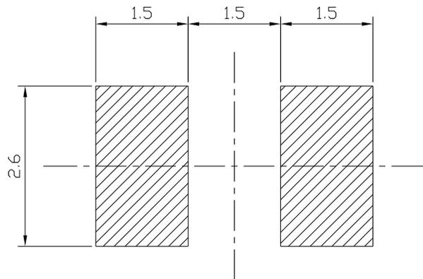
**Note:** Tolerance unless mentioned is  $\pm 0.1\text{mm}$ ; Unit = mm
