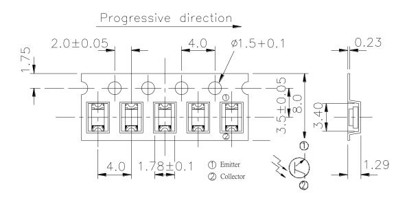
Note: The tolerances unless mentioned are ±0.1mm, Unit: mm
