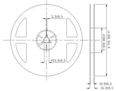
**Note:** The tolerances unless mentioned are ±0.1mm, Unit: mm
