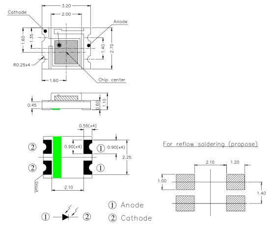
**Notes:** 1.All dimensions are in millimeters 2.Tolerances unless dimensions  $\pm 0.1$ mm
