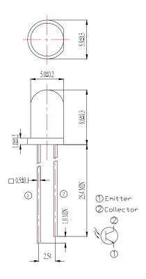
Note: Tolerances unless dimensions ±0.25mm
