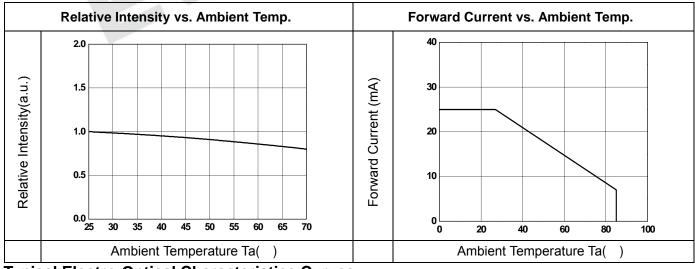
**Typical Electro-Optical Characteristics Curves**
