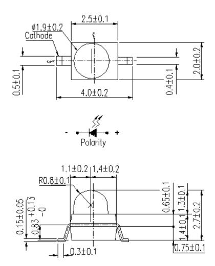
Note: The tolerances unless mentioned are ±0.1, unit=mm.
