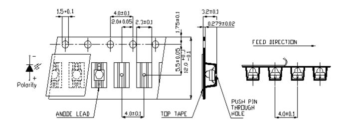
Note: The tolerances unless mentioned are ±0.1, unit=mm.
