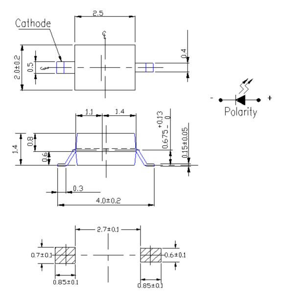
Note: The tolerances unless mentioned are  $\pm 0.1$ , unit=mm.
