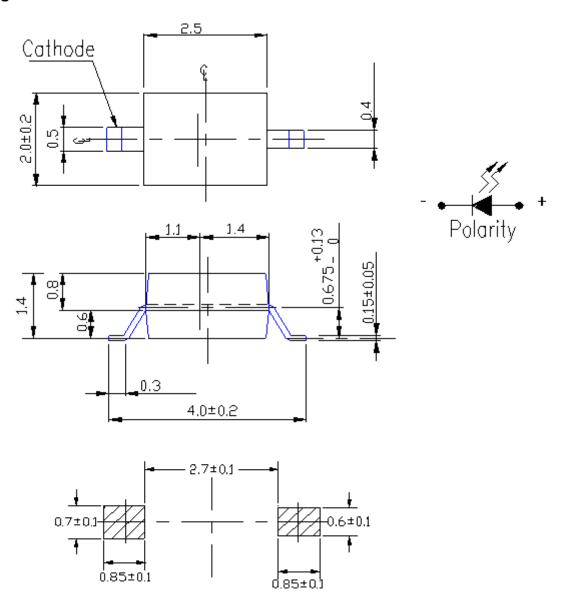
Note: The tolerances unless mentioned are ±0.1, unit=mm.
