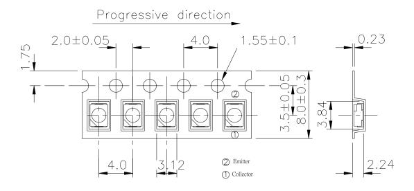
TOLERANCES UNLESS DIMENSION±0.1 ANGLE±0.5 UNIT:mm
