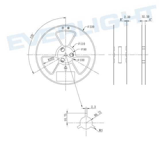
Carrier Tape Dimensions: Loaded Quantity 800 PCS Per Reel
