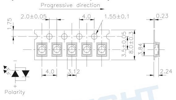
**Note:** Tolerances unless dimension are  $\pm 0.1$ mm, unit = mm.
