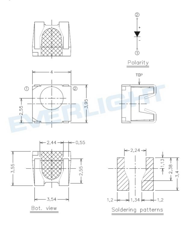
**Note:** Tolerances unless mentioned are  $\pm 0.1$ mm, unit = mm.
