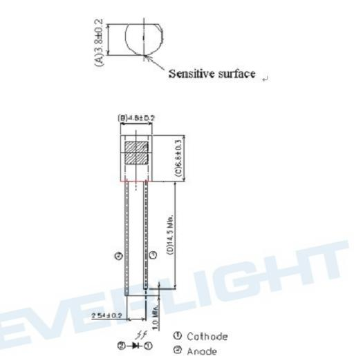
Note: Tolerances unless dimensions ±0.25mm
