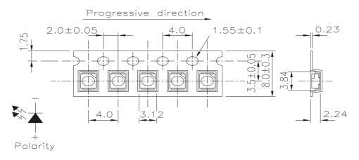
Note: 1.Tolerances unless mentioned ±0.1mm. Unit = mm 2.Minimum packing amount is 250/500/1000/2000 pcs per reel
