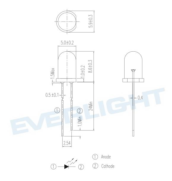
Note: Tolerances unless dimensions ±0.25mm
