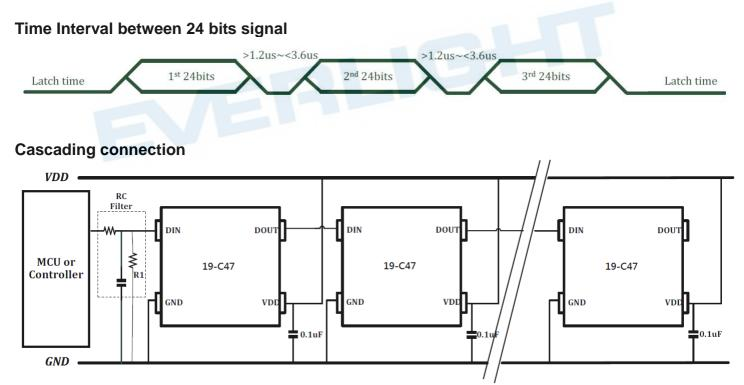
Note1: RC Filter and R1 must be added or reserved on the board for better waveform of signals in different applications.
