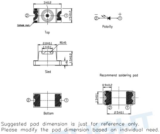
Note: Tolerances unless mentioned ±0.1mm. Unit = mm
