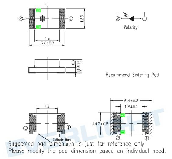
Note: Tolerances unless mentioned ±0.1mm. Unit = mm
