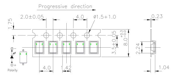
Note: The tolerances unless mentioned is  $\pm 0.1$ mm ,Unit = mm
