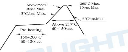
3.2 Reflow soldering should not be done more than two times.
