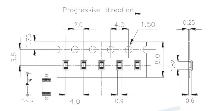
Note: The tolerances unless mentioned is  $\pm 0.05$ mm ,Unit = mm
