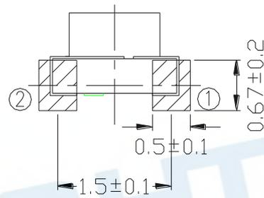
Note: Tolerances unless mentioned  $\pm 0.1$ mm. Unit = mm
