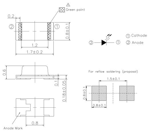
**Notes:** 1.All dimensions are in millimeters 2.Tolerances unless dimensions  $\pm 0.1$ mm
