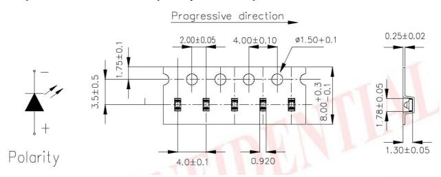
Note: The tolerances unless mentioned is  $\pm 0.1$ mm, Unit = mm
