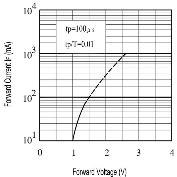
**Typical Electro-Optical Characteristics Curves**
