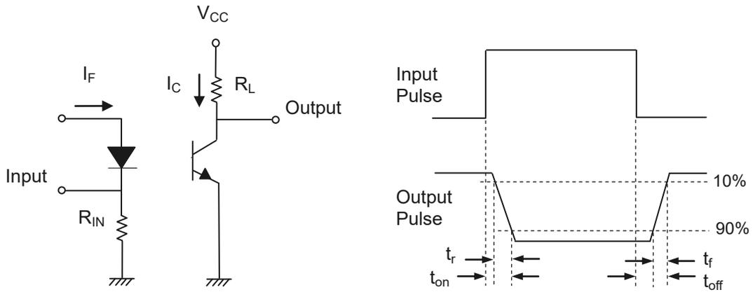
Figure 7. Switching Time Test Circuit & Waveforms
