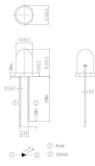
Note: Tolerances unless dimensions ±0.25mm
