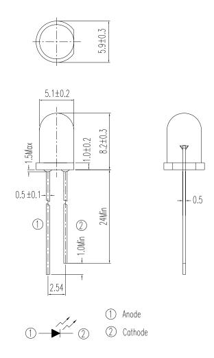
Note: Tolerances unless dimensions ±0.25mm
