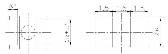
**Note:** Tolerances Unless Dimension ±0.1mm; Unit = mm
