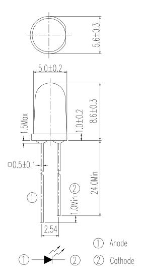
Note: Tolerances unless dimensions ±0.25mm
