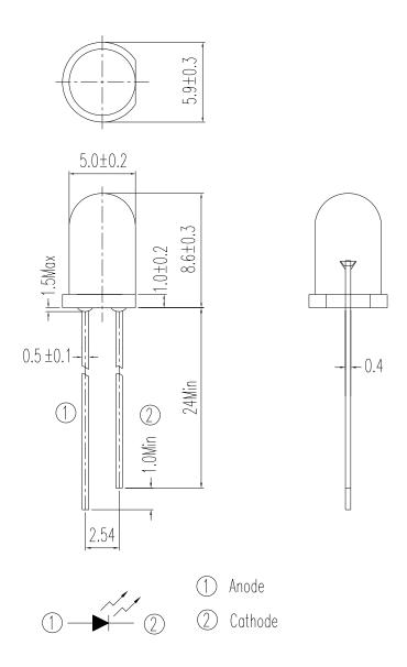
Note: Tolerances unless dimensions ±0.25mm
