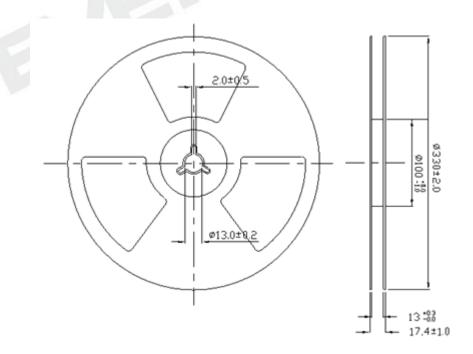
Note: The tolerances unless mentioned is ±0.1mm ,Unit = mm
