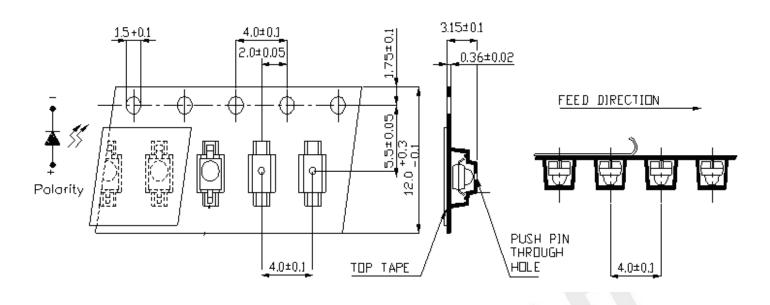
Note: The tolerances unless mentioned is ±0.1mm ,Unit = mm
