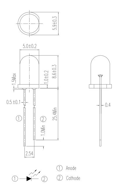
Note: Tolerances unless dimensions ±0.25mm
