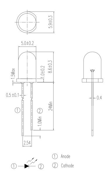
Note: Tolerances unless dimensions ±0.25mm
