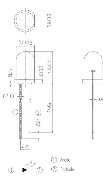
Note: Tolerances unless dimensions ±0.25mm
